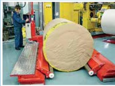
**The Mover's forks are fitted with a lifting device to collect the paper reel directly from the floor.**
