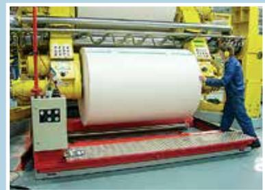
**The paper reel is positioned accurately in the reel changer.**
