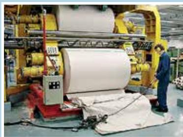
**The reel is raised by a lift table mounted in the floor.**
