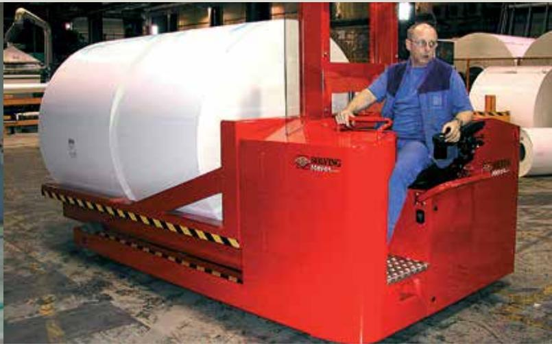
Solving has developed simple and cost effective wheeled pedestrian and stand-on trucks for handling loads weighing 4 to 10 tonnes, such as paper and plastic reels, pallets and containers.
