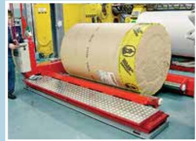
**Integral motorised reel rotators facilitate the unwrapping of reels.**
