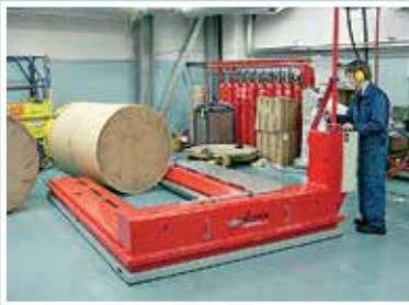
**The paper reel is collected by a U-shaped air film Mover from the storage area.**
