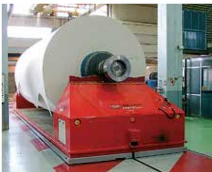
Solving AGV Movers are based on air bearings or wheels, or a combination of both.
